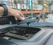
3. Install the base reinforcement plate using the OEM screws. Take note of the screw position in the picture. You may need to adjust this plate later if needed.
