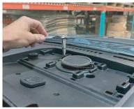
2. Remove the screws holding the dash tray using a 7mm deep socket and pry up the dash tray using plastic dash tools.
