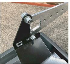
8. Install GPS head unit, lightly tighten all the hardware, swivel the assembly to make sure it functions to your liking and the wiring does not bind.
