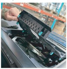
6. Once alignment is confirmed install the swivel base mount using  $4 \times 1/4^{\prime\prime}-20 \times .625^{\prime\prime}$  bolts and washers and the top swivel plate using the plastic washer, and locking lever. We supply a  $3/8^{\prime\prime}$  washer to help align the locking lever to your liking if needed.
