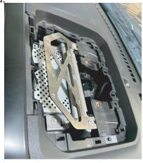
4. Locate the GPS swivel base mount onto the plastic dash tray. Make sure the base mount is centered. Drill 4 x 17/64" holes in the plastic tray. TIP: You can to increase the hole size as you see fit to make final assembly easier. Drill a 3/8" hole for the power wire.
