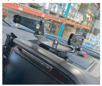
6. Install the billet side plates using the 1/4"x.750" long socket head cap screws, washers, and nylock nuts. Leave loose to allow for final height adjustment.
