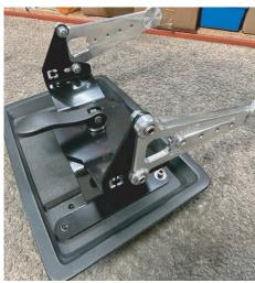
6. Install the billet side plates using the 1/4"x.750" long socket head cap screws, washers, and nylock nuts. Leave loose to allow for adjustment.
