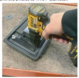
4. Install the base plate using 2 x 1/4" .875" long socket head cap screws and washers. Flip the dash tray and install the reinforcement plate using 2 washers and 2 nylock nuts. Leave nuts loose.
