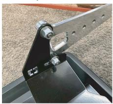
8. Install the complete assembly into the vehicle using the provided phillips head screws. Install the GPS head unit and adjust the height to your liking.
