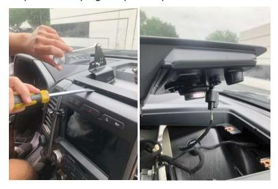
4. Line up the steel base mount for the GPS in the center of the top pocket of the panel. Drill the 4 mounting holes in the panel using a ¼ drill bit for the first holes then open the holes with a 17/64 drill bit.
