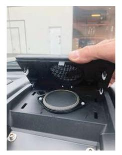
2. Once the speaker cover has been removed, remove the 2 bolts at the back under the speaker cover with a 7mm socket.
