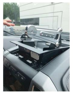
8. Install the GPS head unit and adjust the height to your liking.
