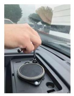
3. Remove the center panel on your dash. Use an automotive trim tool to pry up the front corner of the panel. There are 3 clips on the front of the panel. After the first corner clip comes loose move across and pry up the other 2. The panel will come off front side first then the back will release. Remove the speaker wire plug and pull the panel out.
