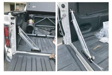
14. Now tighten the 5/16-18 nuts onto the bolts of the cross member. Torque to 14 ft-lbs and you are done.
