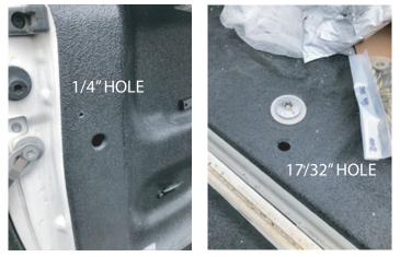
7.Use provided tool to install rivet nuts in the 2 holes. Apply grease between the nut and washers to help assembly. Hold the handle of the tool in place while tightening the nut with a 9/16" wrench. The tool should not spin, only the nut will spin pulling up the nut insert which locks it in place.
